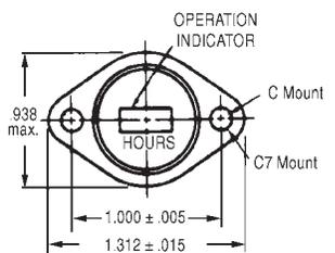
\*When mounting flanged units, it is recommended to distribute the mounting torque evenly across the mounting surface. Each mounting screw should be alternately tightened about one quarter to one half turn until the recommended torque is attained on each screw. The mounting surface should be flat to avoid exerting stress on the body of the unit.
